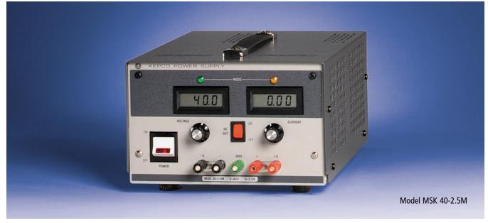
Kepco's MSK linear power supplies provide a selection of five models, offering 100 Watts of stable benchtop power. They use a high gain linear (series pass) stabilizer circuit for low noise output, good stability, and accurate resettability.
