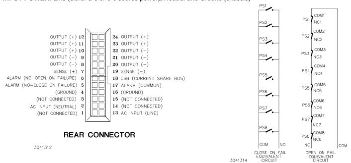
FIGURE 2. REAR CONNECTOR PIN ASSIGNMENTS
