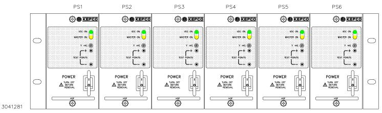
FIGURE 1. HSF 150 WATT POWER SUPPLIES (6) INSTALLED IN RA 19-6B RACK ADAPTER
