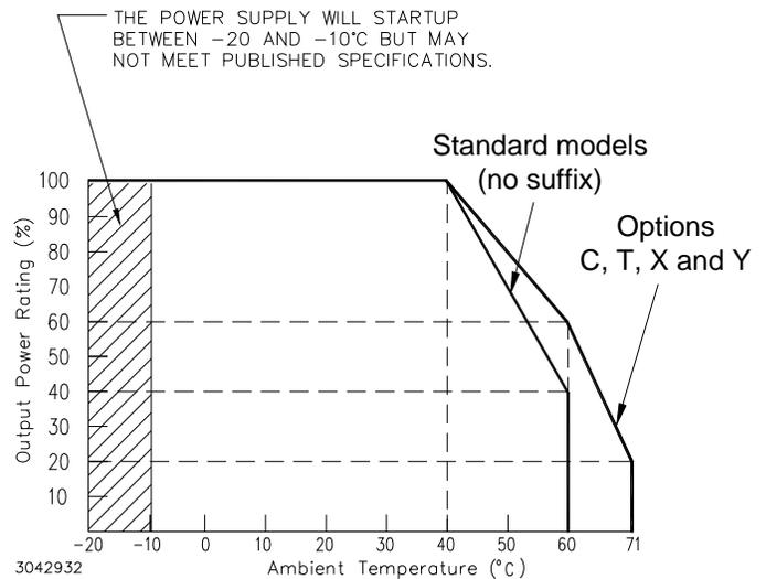
**FIGURE 4. OUTPUT POWER RATING VS. AMBIENT TEMPERATURE**
