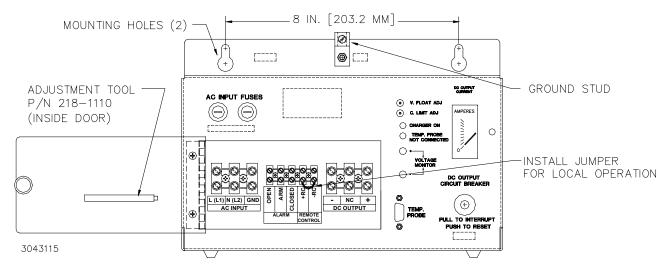
FIGURE 1. 24 VOLT ENGINE START BATTERY CHARGER, FRONT VIEW
