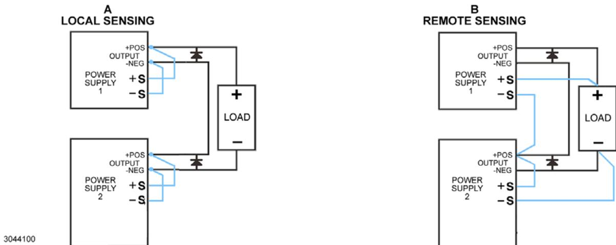
FIGURE 2-20. SERIES CONNECTIONS
