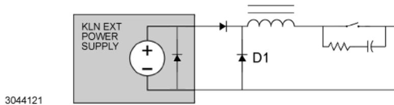
FIGURE 2-15. USING FREE WHEEL DIODE WITH INDUCTIVE LOAD
