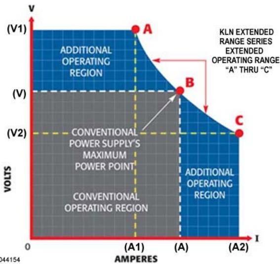
Referring to the adjacent figure, a conventional output power range would require three power supplies to meet the following requirements:
