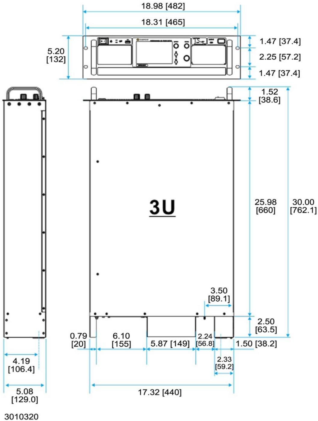
FIGURE 1-4. KLN EXT 5KW, 10KW, 15KW POWER SUPPLY, OUTLINE DRAWING
