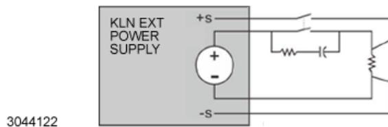
FIGURE 2-16. USING MECHANICAL SWITCH TO TURN OUTPUT ON/OFF
