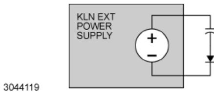
**FIGURE 2-13. USING BLOCKING DIODE WITH HIGH CAPACITANCE LOAD**
