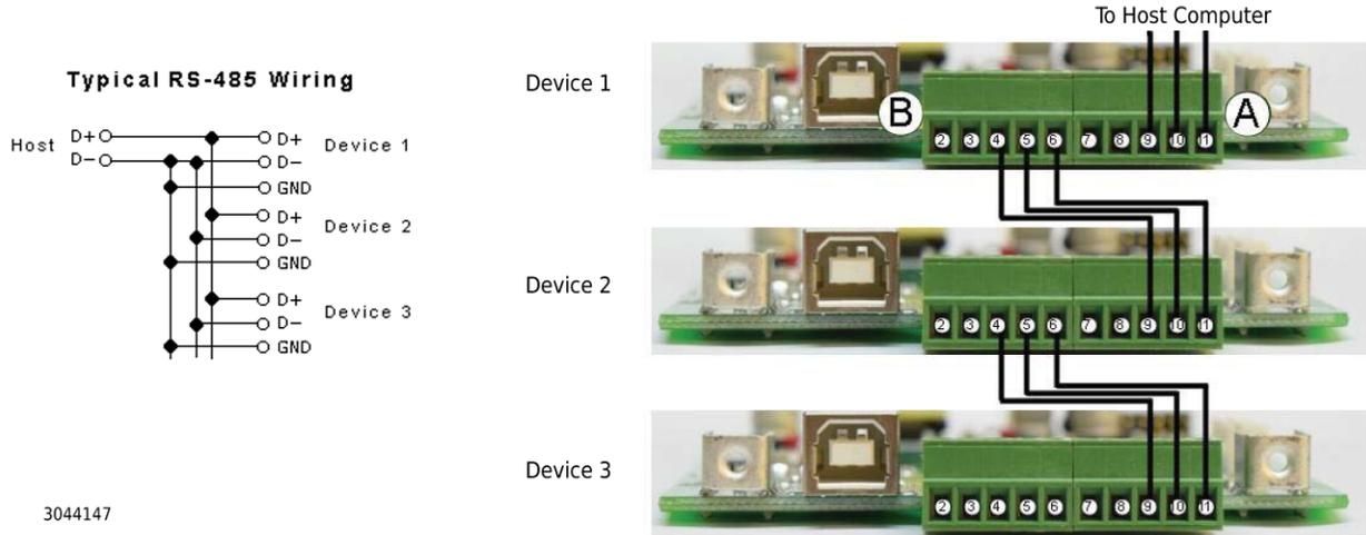
**FIGURE 3-36. RS 485 CONNECTIONS**
