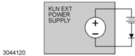
FIGURE 2-14. USING BLOCKING DIODE WITH RECHARGEABLE BATTERY
