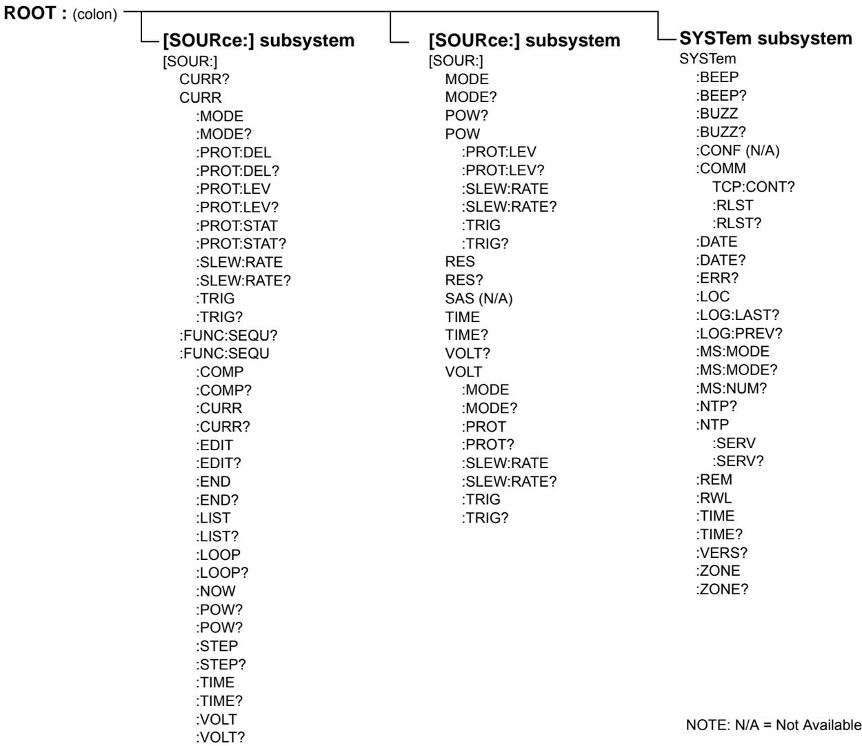
**FIGURE 3-37. TREE DIAGRAM OF SCPI COMMANDS USED WITH KLN POWER SUPPLY (SHEET 2 OF 2)**
