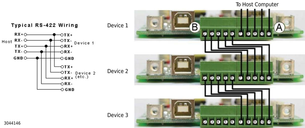
**FIGURE 3-35. RS 422 CONNECTIONS**
