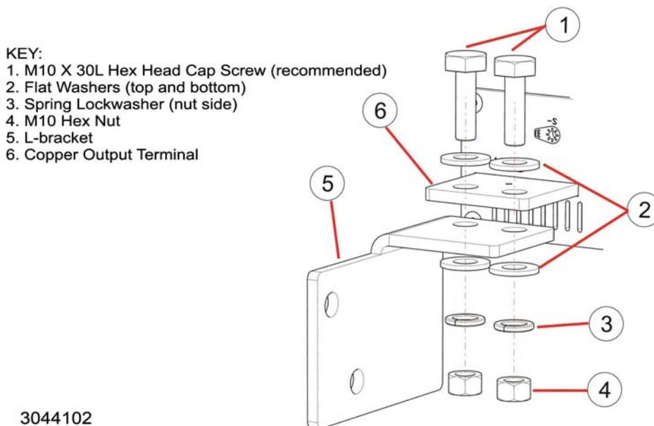
FIGURE 2-22. L-BRACKET INSTALLATION
