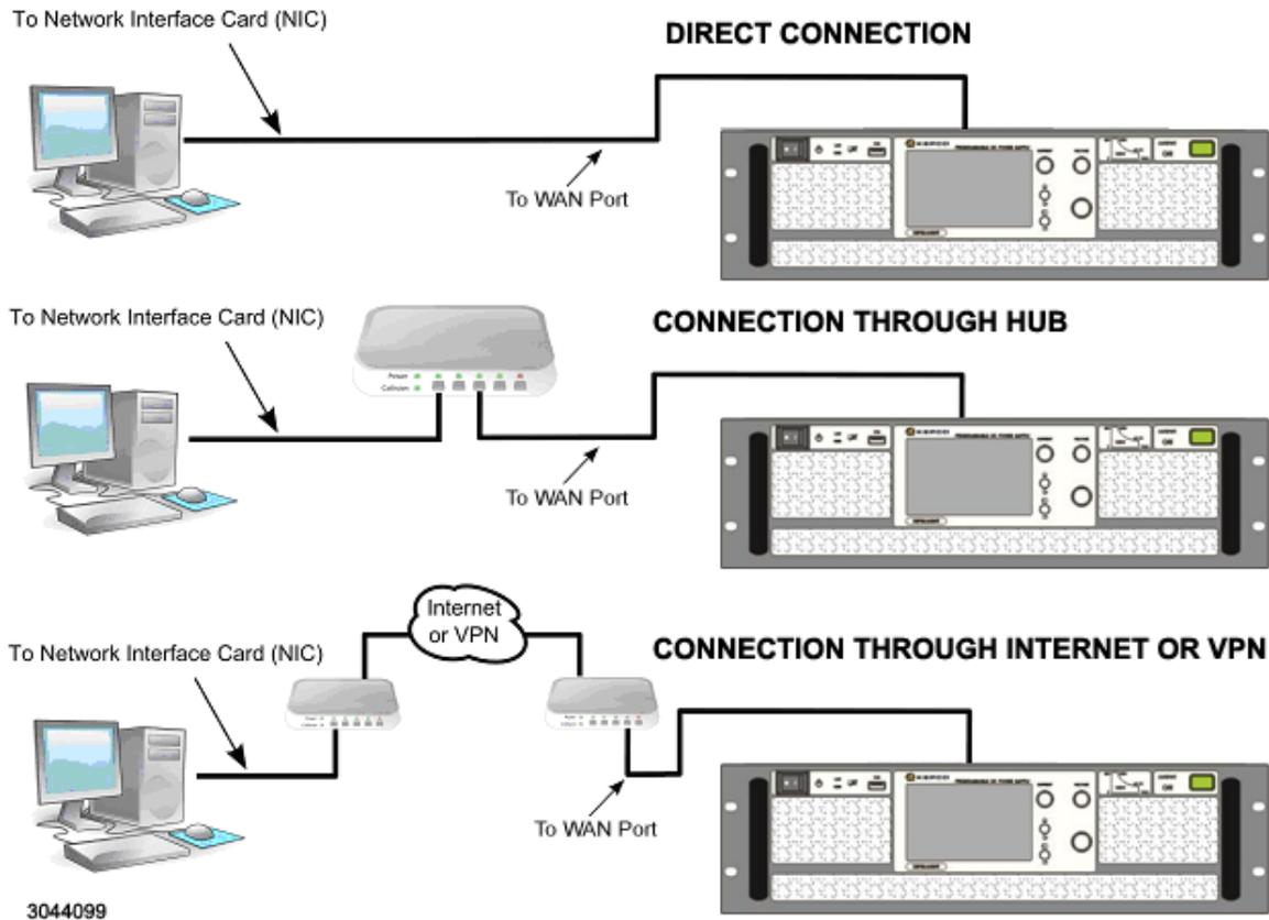
**FIGURE 2-24. LAN CONNECTIONS**
