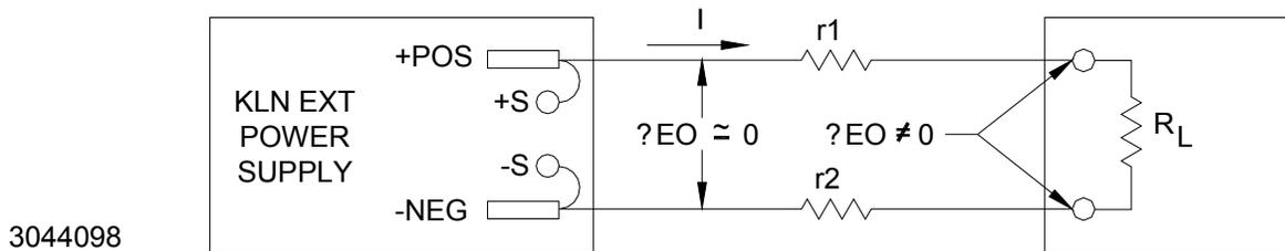
FIGURE 2-10. LOAD WIRE VOLTAGE DROP, EQUIVALENT SCHEMATIC DIAGRAM
