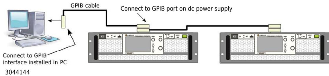
**FIGURE 3-33. GPIB CONNECTIONS**
