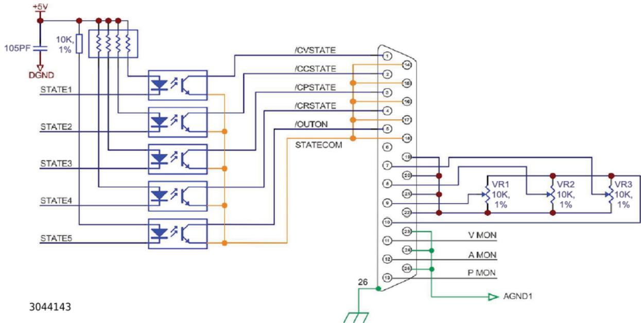
**FIGURE 3-32. ANALOG CONTROL, TYPICAL CONNECTIONS, SCHEMATIC DIAGRAM**
