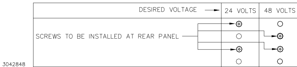
FIGURE 2-1. RA 19-4C-26417 RACK ADAPTER KEYING
