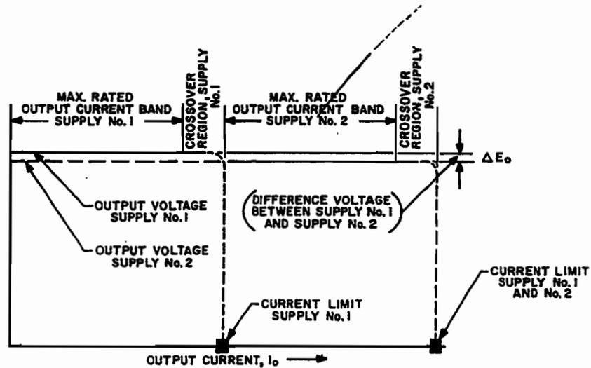
FIG. 3-24 "AUTOMATIC" PARALLEL OPERATION (TWO SUPPLIES).
