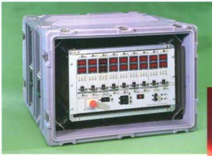
MST power modules are a group of programmable power supplies that are compatible with Kepco's single address, multiple instrument serial control bus. The MST provide precision interactive control in the 200 Watt power class. The housing for MST, RA 55, contains a slot to accommodate an IEEE 488.2 adapter. If not used, a ninth MST power module may be plugged into that slot.
