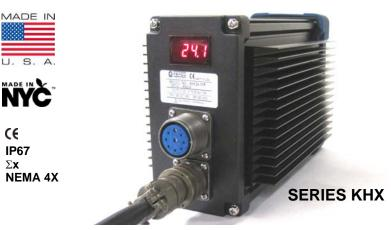
Kepco's sealed KHX power supply modules are ideal for extreme environments applications. The rugged die-cast aluminum housing is water, ice, oil and dust resistant in compliance with IP67 and NEMA 4X standards. The metal case works as an efficient heatsink, allowing full power operation of up to  $+60^{\circ}$ C ambient temperature (no fan required). The unit is shock- and vibration-proof, permitting direct mounting on a machine.
