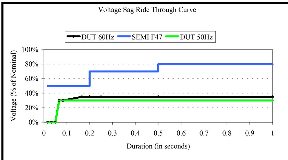
Figure A-4 RKW 48-3.3K SEMI F47 Ride-Through Curve
