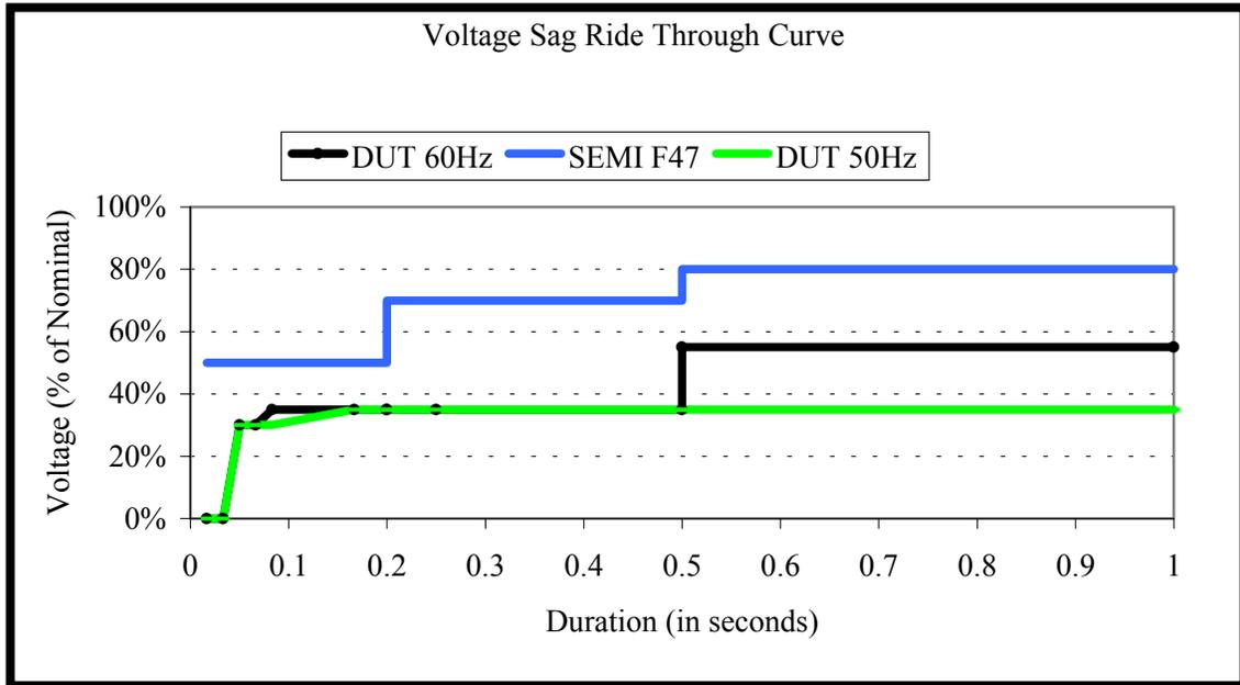
Figure A-3 RKW 24-4.5K SEMI F47 Ride-Through Curve
