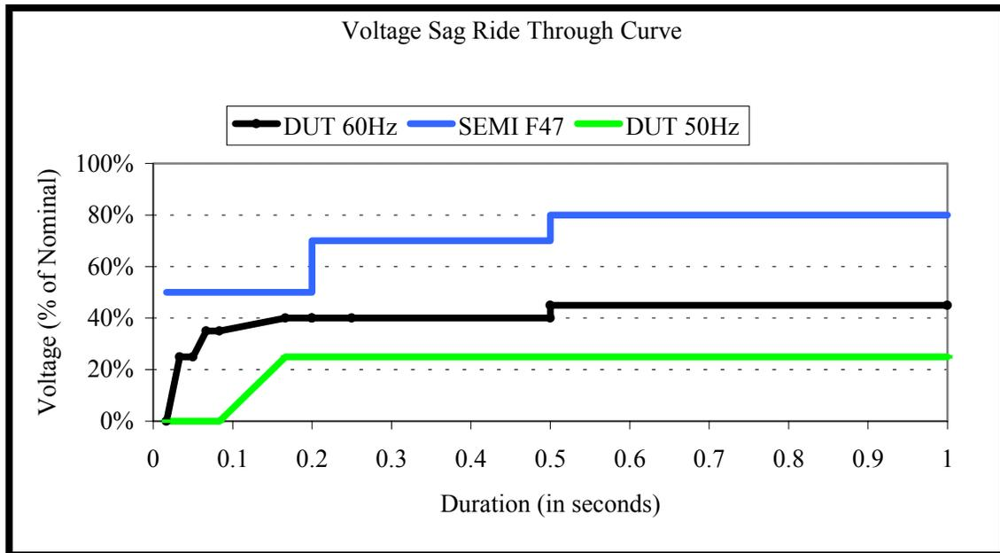
Figure A-2 RKW 12-4.3K SEMI F47 Ride-Through Curve
