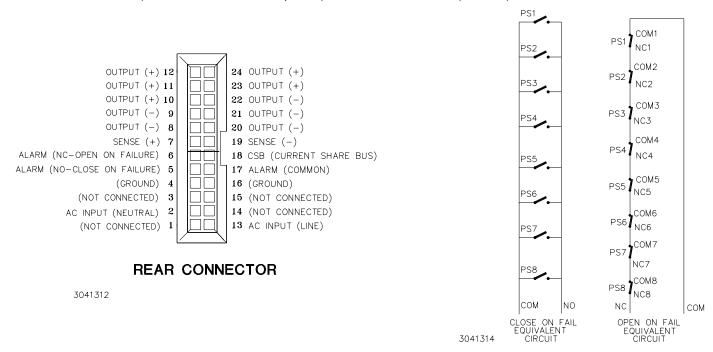
FIGURE 2. REAR CONNECTOR PIN ASSIGNMENTS
