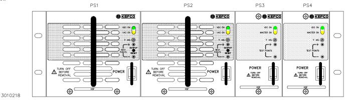
FIGURE 1. RA 19-4B RACK ADAPTER WITH TWO 1/3 RACK AND TWO 1/6 RACK HSF POWER SUPPLIES INSTALLED.
