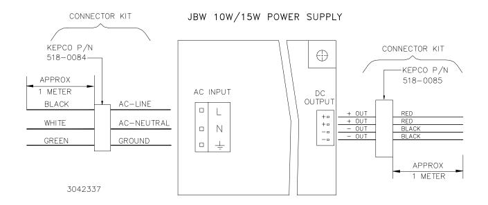
FIGURE 1. CABLE KIT INSTALLATION
