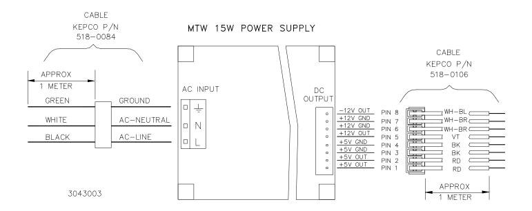
FIGURE 1. CABLE KIT INSTALLATION
