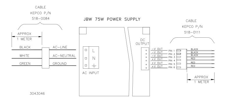
FIGURE 1. CABLE KIT INSTALLATION
