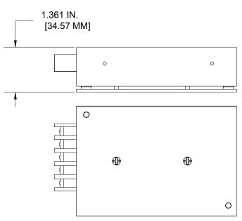
NOTE: MAX PENETRATION OF MOUNTING SCREWS IS 0.24 IN. [6 MM] FROM CASE SURFACE.
