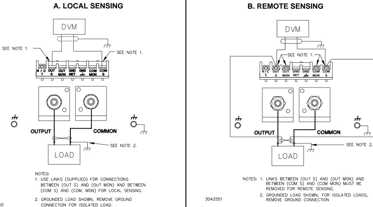
FIGURE 4. LOAD CONNECTION
