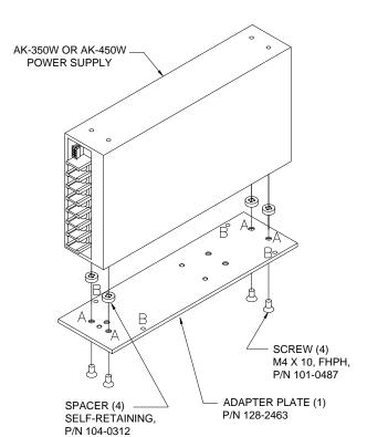
FIGURE 1. ADAPTER PLATE INSTALLATION
