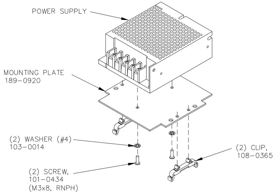
**FIGURE 3. INSTALLATION OF KIT ON POWER SUPPLY**
