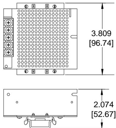
**FIGURE 4. POWER SUPPLY WITH KIT INSTALLED, OUTLINE DIMENSIONS**
