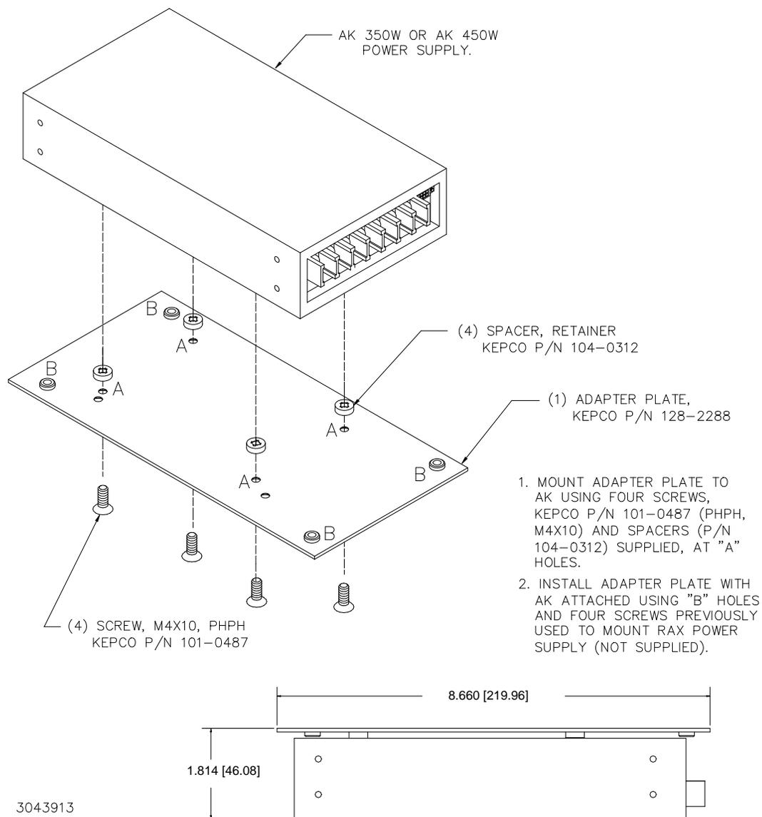
**FIGURE 1. ADAPTER PLATE INSTALLATION**
