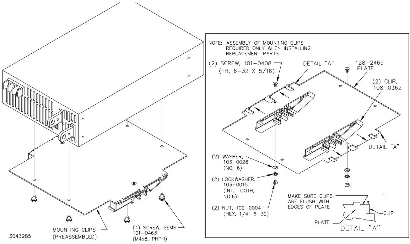
**FIGURE 3. INSTALLATION OF KIT ON POWER SUPPLY**
