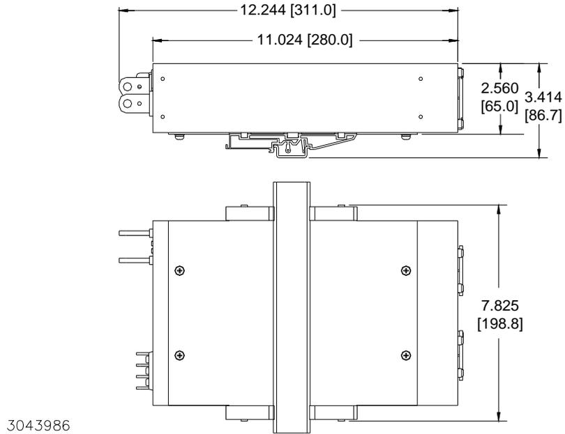
**FIGURE 4. POWER SUPPLY WITH KIT INSTALLED, OUTLINE DIMENSIONS**
