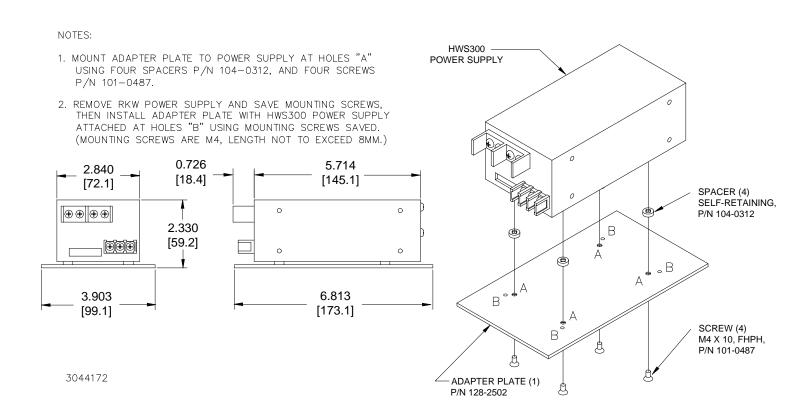
FIGURE 1. ADAPTER PLATE INSTALLATION
