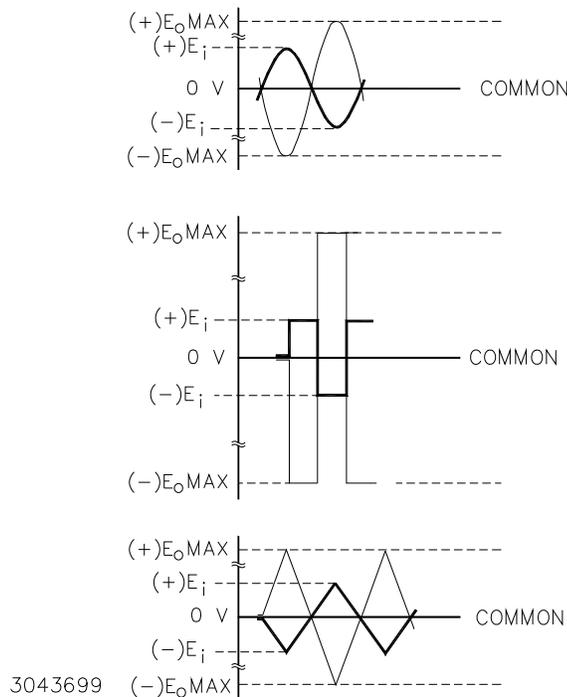
**FIGURE 3-1. GRAPHS OF POSSIBLE INPUT/OUTPUT WAVESHAPES**
