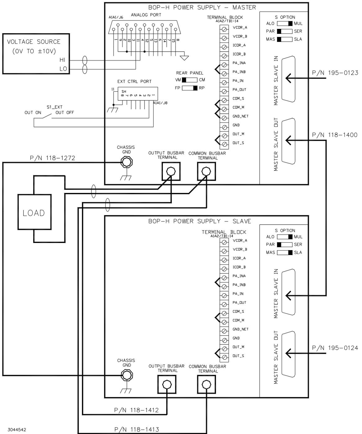
NOTE: Consult factory for configurations requiring more than two units in parallel.
