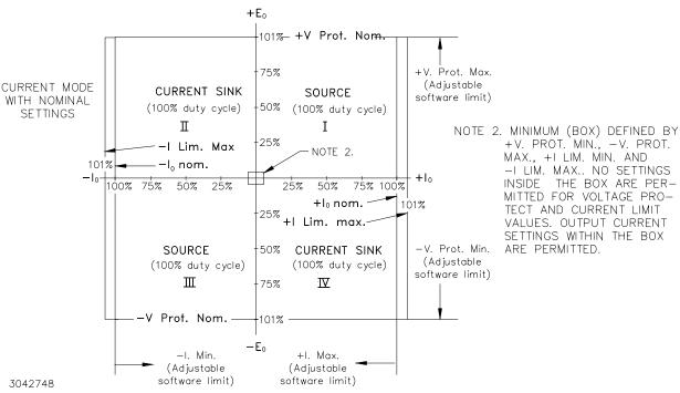
FIGURE 1-2. BOP OUTPUT CHARACTERISTICS
