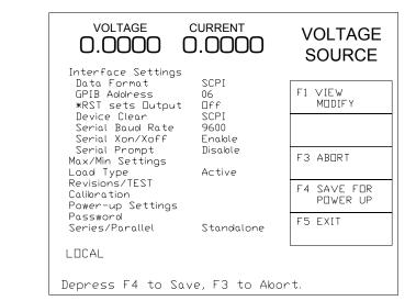
NOTE: F3 AND F4 ARE ONLY VISIBLE IF A CHANGE HAS BEEN MADE TO A SUBMENU.
