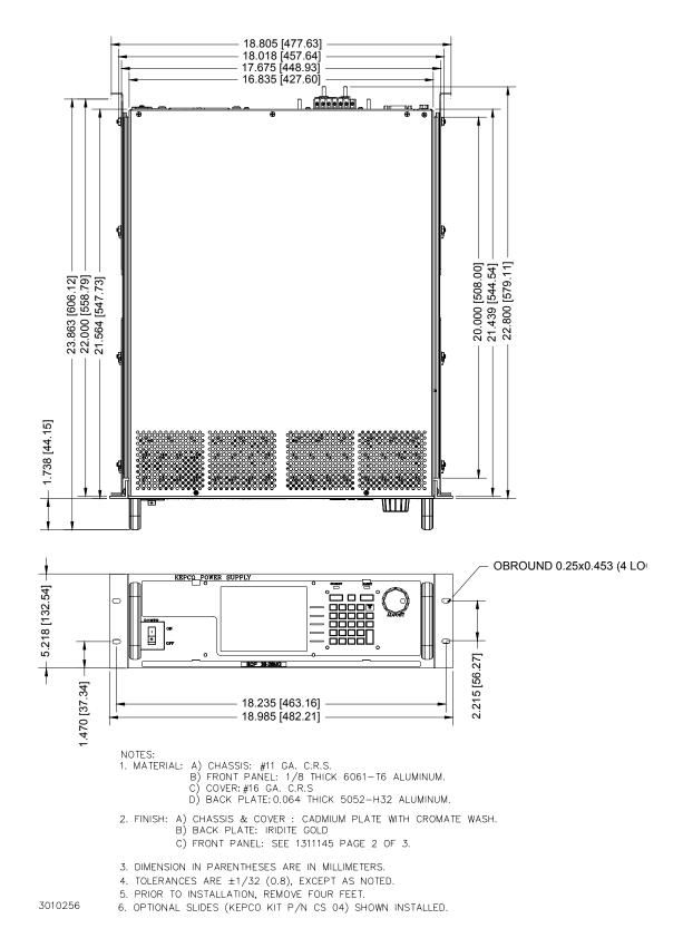
FIGURE 1-1. 1000W BOP POWER SUPPLY, OUTLINE DRAWING (SHEET 1 OF 2)
