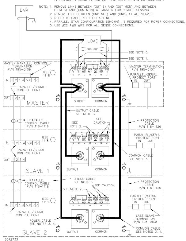
FIGURE 2-5. PARALLEL CONFIGURATION, REMOTE SENSING, TYPICAL
