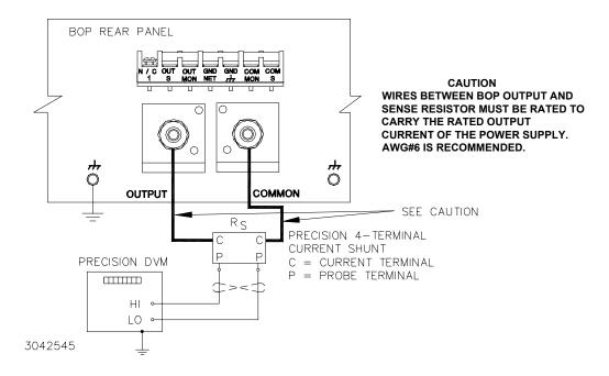
FIGURE 4-2. CURRENT SHUNT (SENSE RESISTOR) CONNECTIONS
