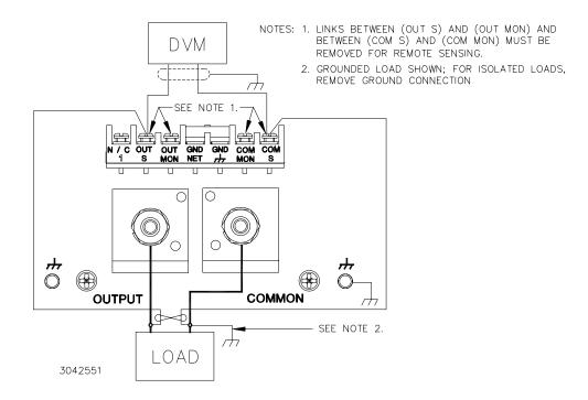
FIGURE 2-3. LOAD CONNECTIONS, REMOTE SENSING
