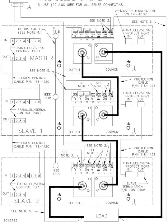
FIGURE 2-7. SERIES CONFIGURATION, REMOTE SENSING, TYPICAL
