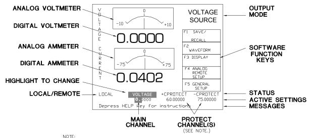
WHEN SET TO BIPOLAR, ONLY ONE PROTECTION FIELD IS DISPLAYED.
