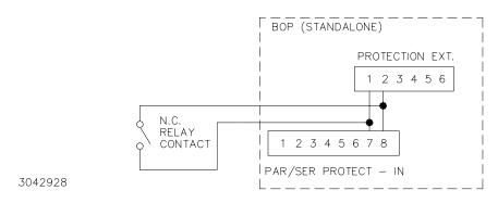
FIGURE 3-13. REMOTE SHUTDOWN USING INTERNAL POWER, STANDALONE UNITS
