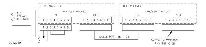
FIGURE 3-14. REMOTE SHUTDOWN USING INTERNAL POWER, MULTIPLE UNITS,
