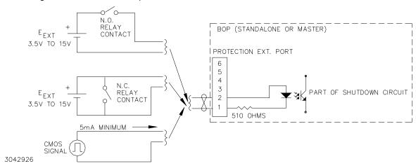
FIGURE 3-12. REMOTE SHUTDOWN USING EXTERNAL POWER, STANDALONE OR MULTIPLE UNITS
