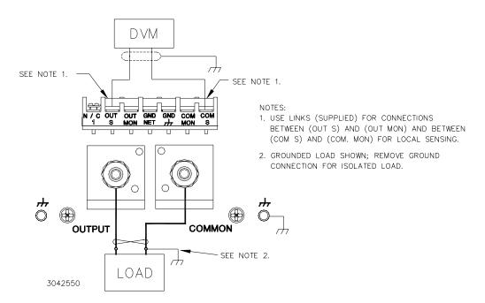
FIGURE 2-2. LOAD CONNECTIONS, LOCAL SENSING
