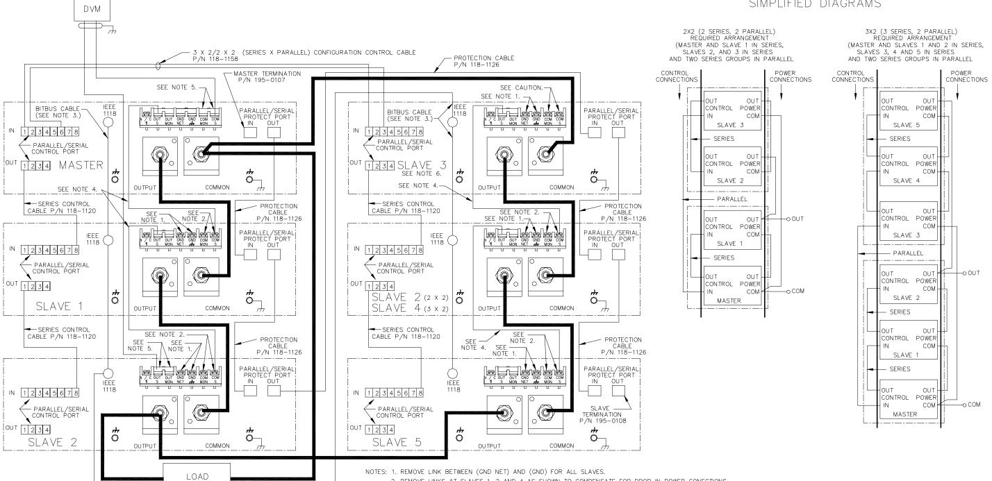
CAUTION: REMOVE LINK BETWEEN (COM S) AND (COM MON) AT SLAVE 3 TO PREVENT DAMAGE TO THE BOP AND TO MAINTAIN SYSTEM ACCURACY.
