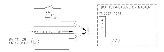
FIGURE 3-15. REMOTE STANDBY, STANDALONE OR MULTIPLE UNITS
