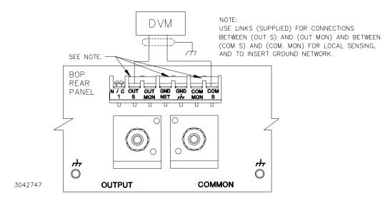
FIGURE 4-1. CALIBRATION SETUP
