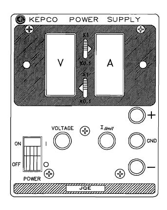
FIG. 2-3 CONTROLS AND TERMINATIONS, JQE 1/4 RACK GROUP FRONT
