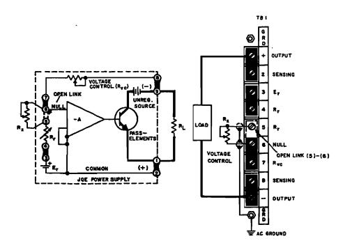
FIG. 3-8 REMOTE CONDUCTANCE PROGRAMMING
