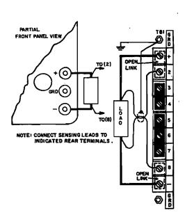
FIG. 3-3 LOAD CONNECTION WITH ERROR SENSING.
