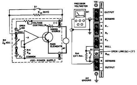
FIG. 3-5 CONNECTIONS FOR PRECISION PROGRAMMING RATIO ADJUSTMENT
