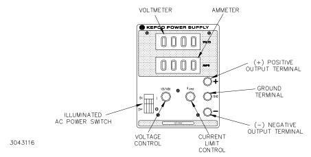
FIGURE 3. FRONT PANEL VIEW OF JQE QUARTER RACK DM (DIGITAL METER) MODELS
