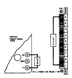
FIG. 3-2 LOAD CONNECTION
