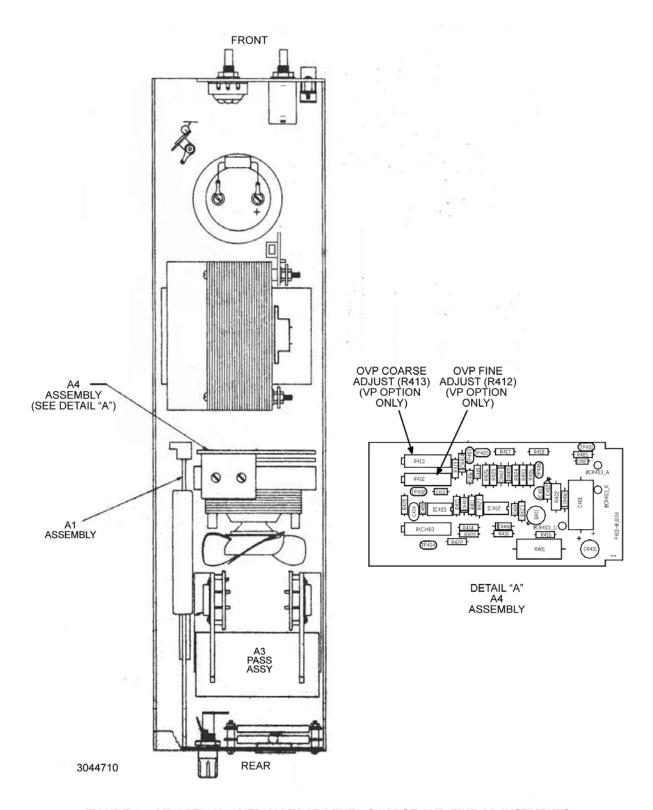
FIGURE 1. VP OPTION: OVERVOLTAGE LEVEL COARSE AND FINE ADJUSTMENTS
