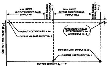
FIG. 3-13 PARALLEL OPERATION, JQE SUPPLIES.
