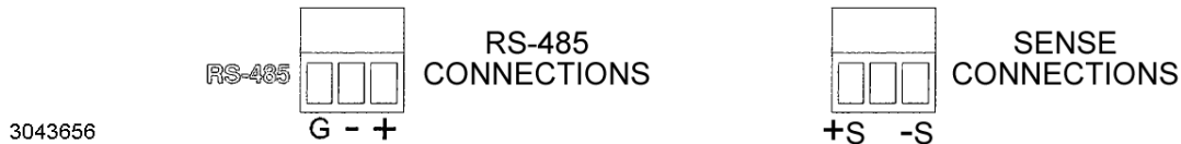
FIGURE 2-5. RS-485 PORT AND SENSE CONNECTIONS
