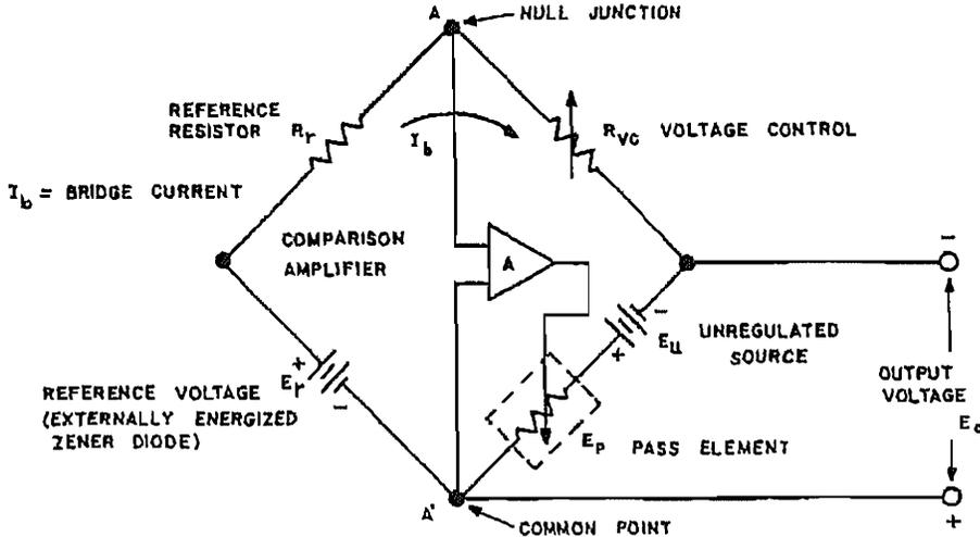
FIG. 3-4 KEPCO POWER SUPPLY AND COMPARISON BRIDGE CIRCUIT.
