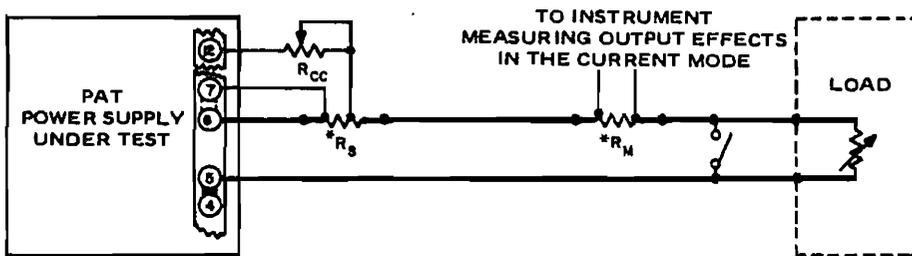
C) OUTPUT EFFECT MEASUREMENT (CURRENT).
