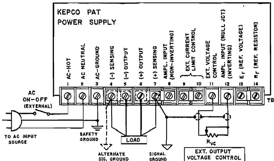
FIG. 3-2 LOAD CONNECTION WITH REMOTE ERROR SENSING.
