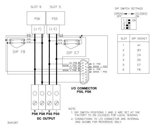
FIGURE 2-2. INDEPENDENT OPERATION, LOCAL SENSING FOR PS5 AND PS6 USING INTERNAL DIP SWITCHES, SIMPLIFIED DIAGRAM
