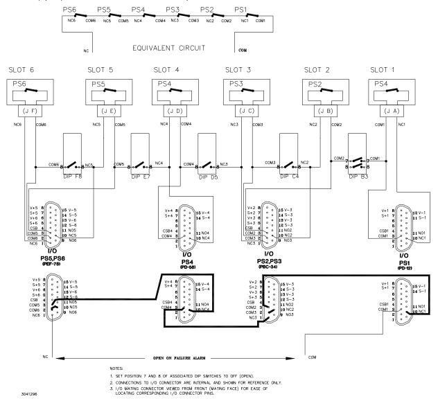
FIGURE 2-15. OPEN ON FAILURE ALARM CONFIGURATION USING EXTERNAL WIRING AT I/O MATING CONNECTOR, SIMPLIFIED DIAGRAM
