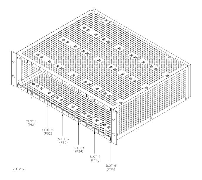
FIGURE 1-1. RA 19-6B RACK ADAPTER
