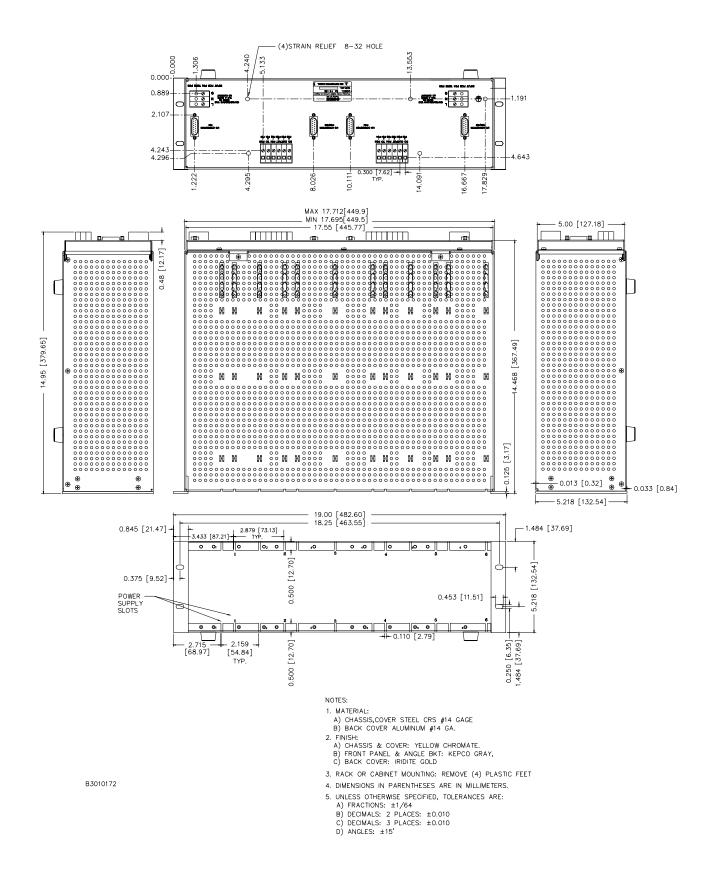
FIGURE 1-5. MECHANICAL OUTLINE DRAWING, RA 19-6B RACK ADAPTER
