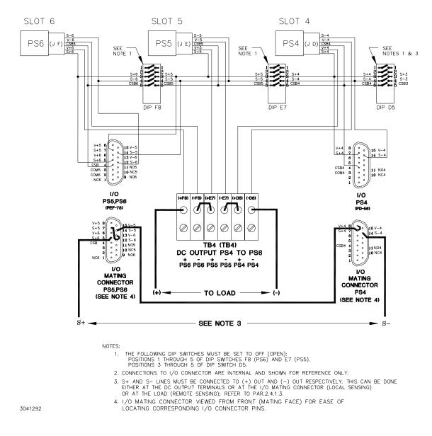
FIGURE 2-11. SERIES CONFIGURATION, SIMPLIFIED DIAGRAM
