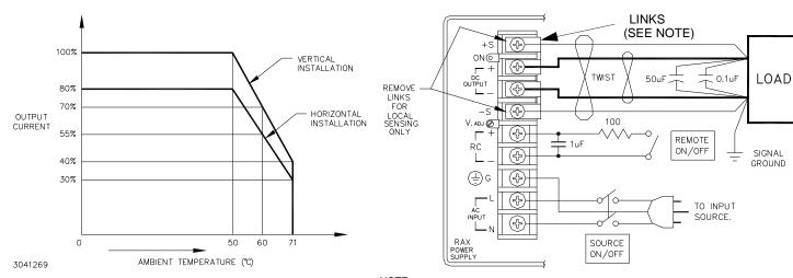
NOTE: THE SENSE LEADS MUST NEVER BE DISCONNECTED FROM THE OUTPUT. IF THE SENSE LEADS ARE ALLOWED TO FLOAT FREE OF THE OUTPUT, THE OUTPUT VOLTAGE WILL RISE TO THE OVERVOLTAGE POINT AND THE UNIT WILL SHUT DOWN.
