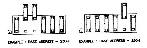
Figure 2-2. Base Address Jumper Examples
