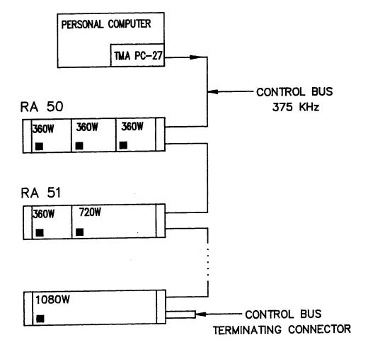
Figure 3-1. TMA PC-27 To MAT Power Module, Interface
