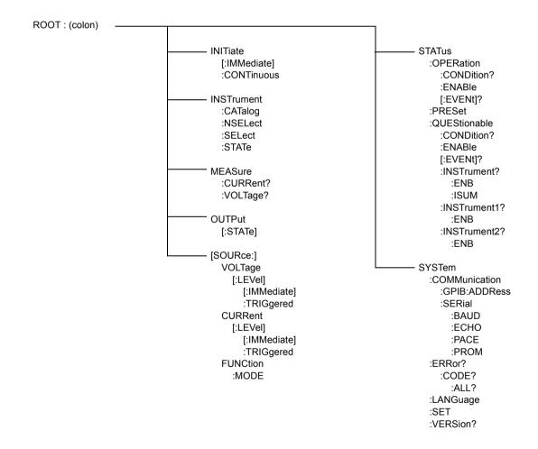
FIGURE 3-4. TREE DIAGRAM OF SCPI COMMANDS USED WITH TMA VXI-27 CONTROLLER
